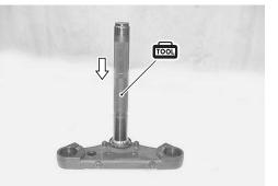
• Apply grease to the upper and lower bearings before remounting the steering stem.
