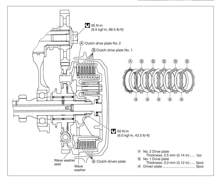
• Install the wave washer seat ① and the wave washer ②.
