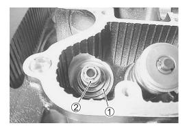
Insert the valves, with their stems coated with high quality molybdenum disulfide lubricant (SUZUKI MOLY PASTE) all around and along the full stem length without any break.
