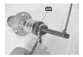
• Install the new bearing with the special tool.
