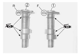
• Align the arrow marks on the front and rear camshafts so it is parallel with the surface of the cylinder heads.
