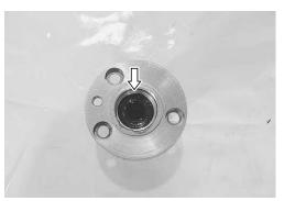
• Remove the mechanical seal ring (3) and rubber seal (4).
