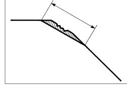
• Insert the solid pilot ① (09916-24450: N-100-5.52) with a slight rotation. Seat the pilot snugly. Install the 45° cutter, attachment and T-handle.
