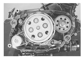
• Install the clutch cover and tighten the bolts.
