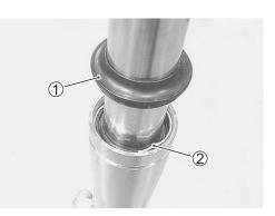
• Remove the oil seal by slowly pulling out the inner tube.
