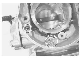
• Remove the casting valve cover.
