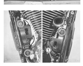
• Remove the frame down tube.
