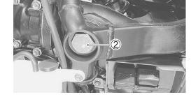
• Remove the tapered roller bearings.
