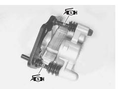
• Tighten the brake caliper mounting bolts (1), and brake hose union bolt 2 to the specified torque.
