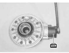
• Apply a small quantity of the THREAD LOCK "1303" to the final drive bevel gear coupling nut.
