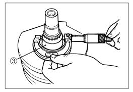
• Measure the crankshaft journal bearing I.D. ① by using the special tool.
