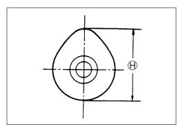
If the camshaft journal oil clearance measured exceeds the limit, measure the outside diameter of camshaft.
