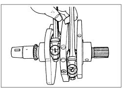
• Remove the caps and measure the width of compressed plastigauge with envelope scale. This measurement should be taken at the widest part.
