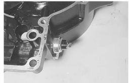
When installing the switch, apply SUZUKI BOND "1207B".
