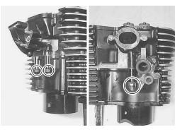
• Remove the cylinder head bolt and nut. (Rear cylinder)
