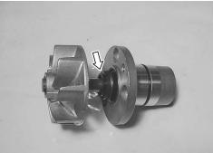
• Install the new mechanical seal with a suitable size socket wrench and the special tool.
