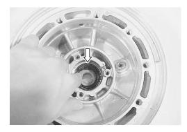
• Install the needle roller bearing for the final driven bevel gear into the final gear case with the special tool.
