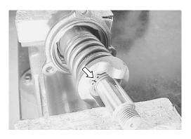
• Remove the cam dog 1 and damper spring 2.
