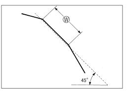
• After the desired seat position and width is achieved, use the 45° cutter very lightly to clean up any burrs caused by the previous cutting operations.
