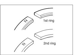
• Position the gaps of the three rings as shown. Before inserting each piston into the cylinder, check that the gaps are so located.
