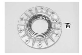
• Apply SUZUKI BOND "1207B" to the mating surface of the final gear case and final gear bearing case.
