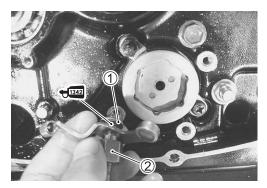
• Install the cam driven gear ① after installing the springs, pins and gearshift pawls.
