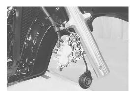
• Remount the front fork and tighten the front fork lower clamp bolts temporarily.
