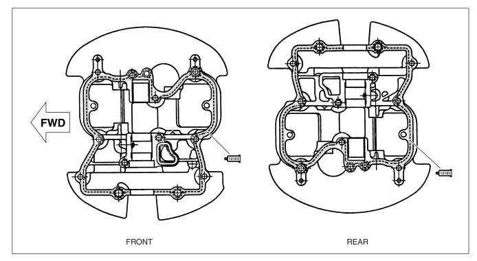
• Lightly tighten the cylinder head cover bolts diagonally, and then if everything is satisfactory, tighten securely with a torque wrench to the specified torque.
