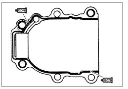
• Tighten the secondary gear case bolts to the specified torque.
