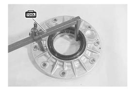
• Remove the bearing retainer screws, using an impact driver set.
