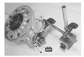
If the backlash is not within the specification, adjust the shim thickness as follows:
