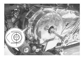
Inspect the No.2 engine's valve clearance as the same manner above.
