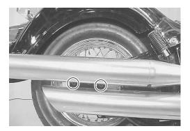
• Remove the No. 1 exhaust pipe and the No. 2 muffler.
