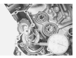
• Adjust the dial gauge so that it touches the secondary drive bevel gear cam dog; hold the driven bevel gear securely, and turn the drive bevel gear in each direction, reading the total backlash on the dial gauge.
