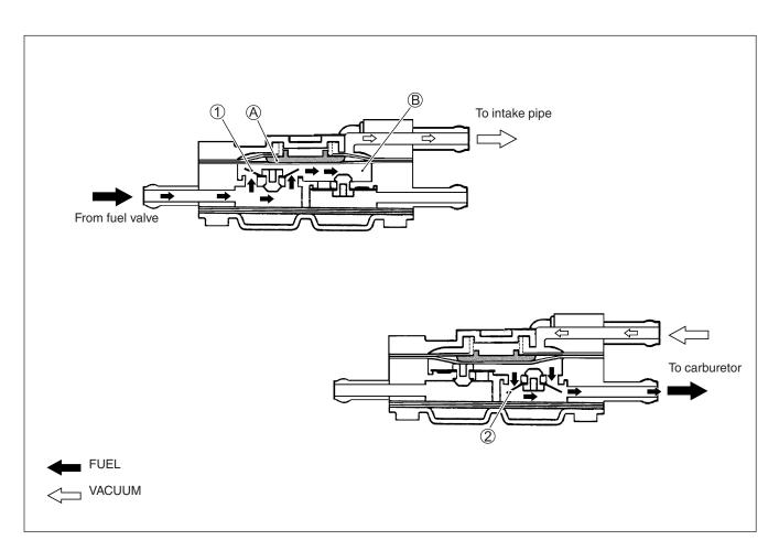
If the fuel pressure in the chamber of carburetor side is too high, the return valve ③ is opened so that the fuel pressure is released to the chamber of fuel cock side.
