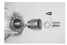
• Tighten the nut to the specified torque with the special tool.
