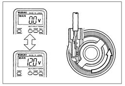
Under above condition, by rotating the drive lugs of speed sensor slowly, the tester reading voltage relatively changes (0V  $\rightarrow$  12V or 12V  $\rightarrow$  0V). If the tester reading voltage does not change, replace the speed sensor with a new one.
