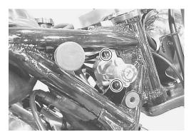
Inspect each switch for continuity with a tester. If any **STARTER BUTTON** abnormality is found, replace the respective switch assemblies with new ones.
